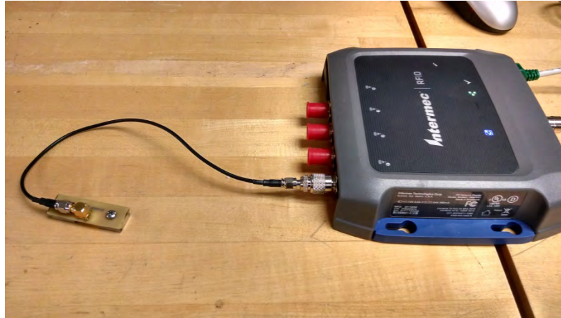
Figure S10. Custom touch probe connected to commercially available RFID reader
